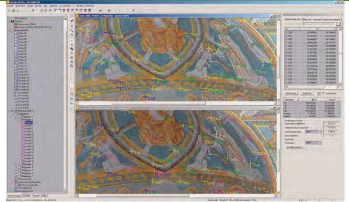
Castle Katzenstein, Chapel Relative and absolute model orientation with automated point detection
